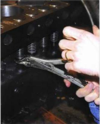
After you are sure the valve will fit properly, install the spring. I find it easier to place the retainer on the end of the spring, and then rest the whole assembly on the spring compressor. I use the tool for leverage, pushing up to get the retainer onto the top of the lifter.
